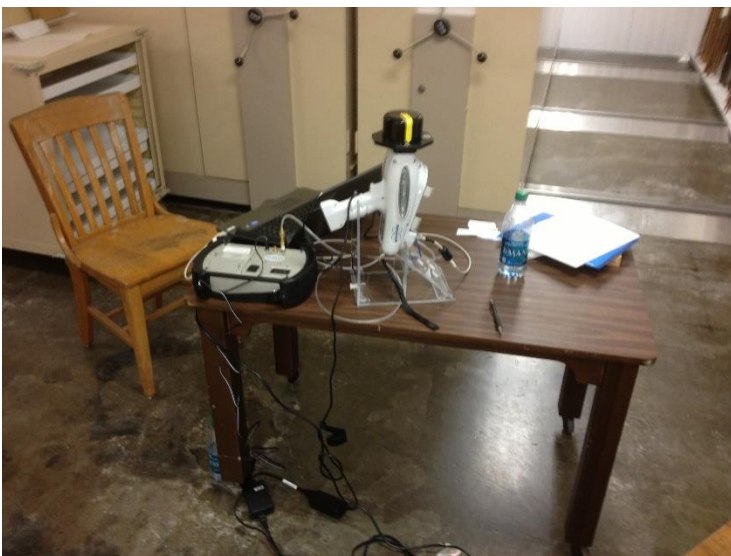
A portable X-ray fluorescence unit set up in the artifact vault at the Texas Archeological Research Laboratory in Austin to analyze Texas chert Clovis artifacts. The artifact stage is the black part sitting on top of the XRF source/detector unit.
