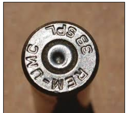
Figure 3. A firing pin imprint on the primer of a .38 Special caliber revolver cartridge case. Firearms, Toolmarks, And Impressions.
